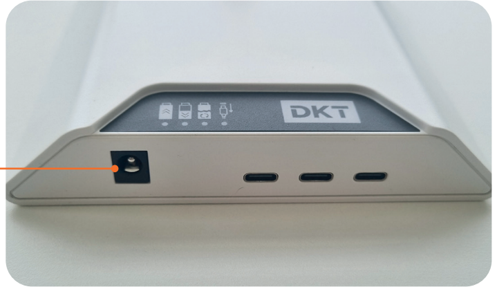
Battery backup unit
