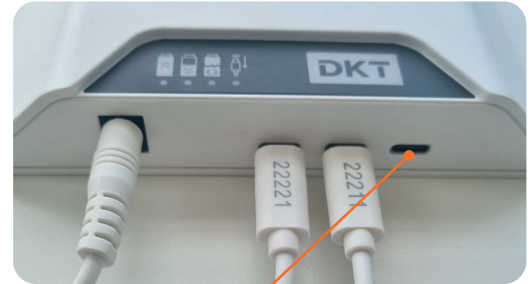
Battery backup unit
