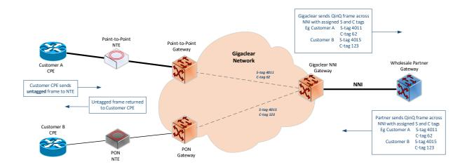
**IMPORTANT:** The wholesale partner is responsible for adhering to the NNI specification in this document. The only device to connect to the NNI must be the Partner QinQ termination device. Loop testing must NOT be performed on the Gigaclear Network, as this will disrupt services for other customers. Breaking these rules will result in Gigaclear shutting down the NNI termination point facing the individual NNI partner.
