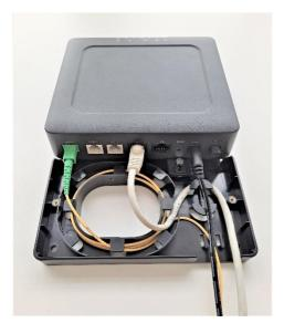
**Note**: Only the 10GE port is enabled on the ONT and must be used for connection to the CPE
